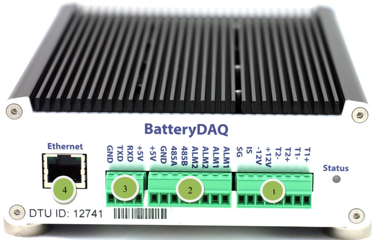
Connector 1: Current Sensor and Temperature Sensors
